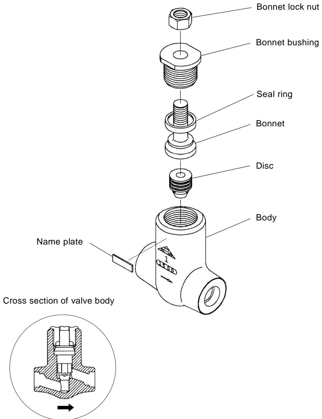
Figure 2.3 Typical Example for Class 150 Check Valve
