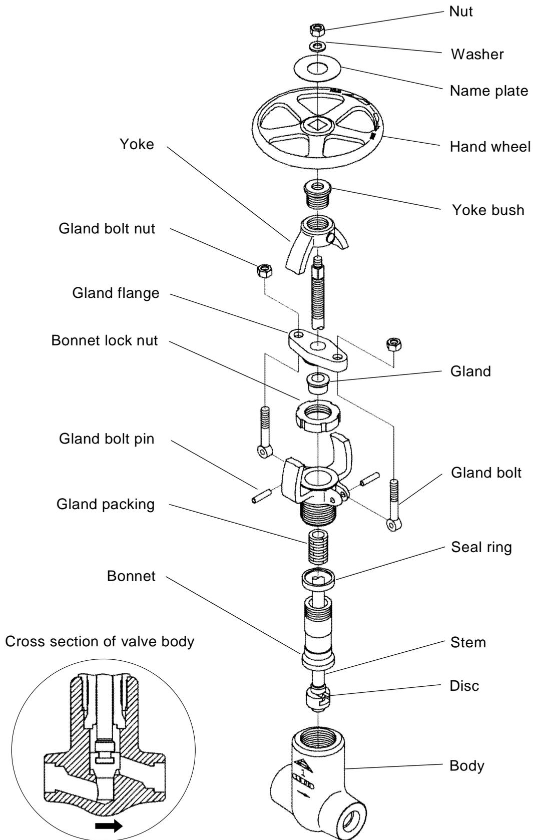
Figure 2.2 Typical Example for Class 1500 Globe Valve
