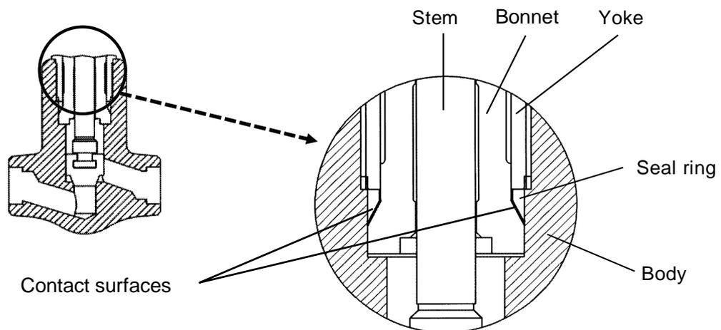
Figure 1.1 Detail of the Contact Surfaces between the Seal Ring and the Bonnet for Pressure Seal Bonnet Type (Globe Valve)
